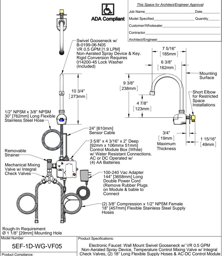
ASME A112.18.1 / CSA B125.1 NSF 61 - Section 9 NSF 372 (Low Lead Content) ANSI A117.1 (ADA) UL 1951
