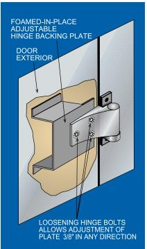
Unique adjustable hinge backing plates in every entry door ensure a proper fit during installation and allow for any necessary future adjustments without removal of the door or its frame.
