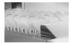
Result: more volume and versatility, quicker work. Its speed is easily adjustable for the type of ware, soiled condition, or workforce requirements. It runs at 4.0 - 8.5 feet per minute.
