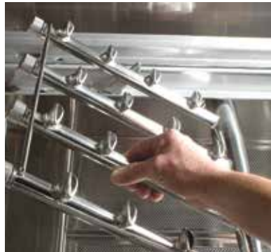
One-Piece Cast Stainless Steel Spray Assembly
