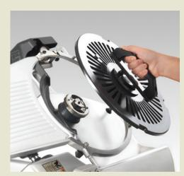
> Removable-knife feature. On select models (see back page), our patented knife comes with a patented kniferemoval tool. With the knife safely removed, sanitation is improved, too, thanks to easily accessible surfaces.
