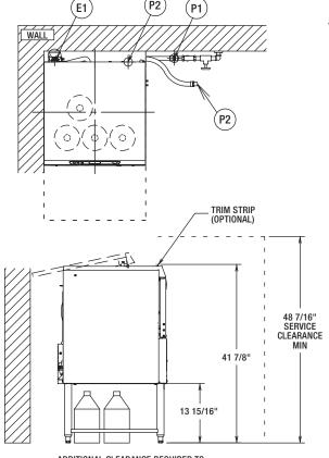
ADDITIONAL CLEARANCE REQUIRED TO SLIDE UNIT FORWARD FOR SERVICE ONLY
